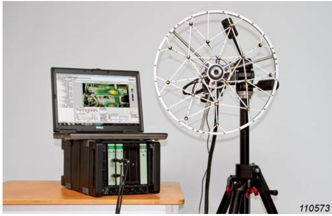
Fig. 23 Front Panel UA-2112 being used in an array application
